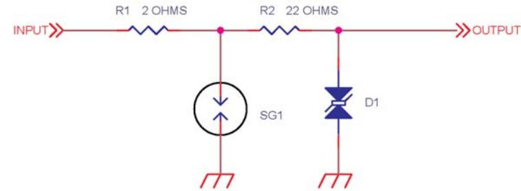
Normally, the gas discharge tube (GDT) does not fire unless a transient over 350 volts is encountered. This action will preserve the useful life of the GDT.
