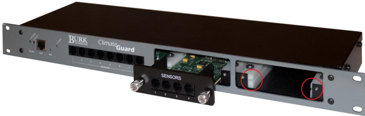
Installing expansion modules; card guides are circled in red
