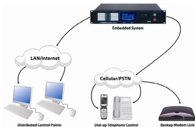
Fig. 2: Server-Client Topology. An embedded system remains connected to the outside world without requiring a central server or computer for data management. Client-side access to the system is flexible.
