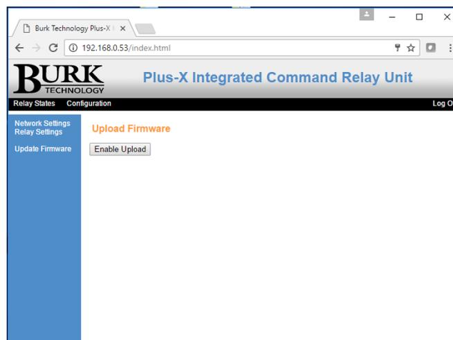
Click **Enable Upload** to prepare the Plus-X ICRU to receive the new firmware.
